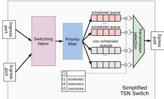
Figure 1. Simplified representation of an IEEE 802.1Qbv-capable switch.
