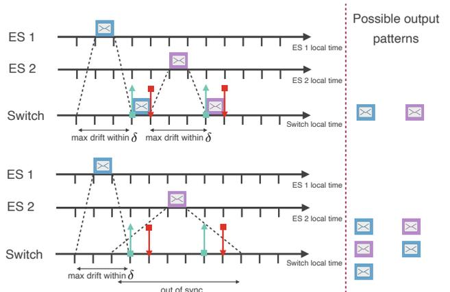
Figure 2. Non-deterministic frame transmission for out-of-sync devices.
