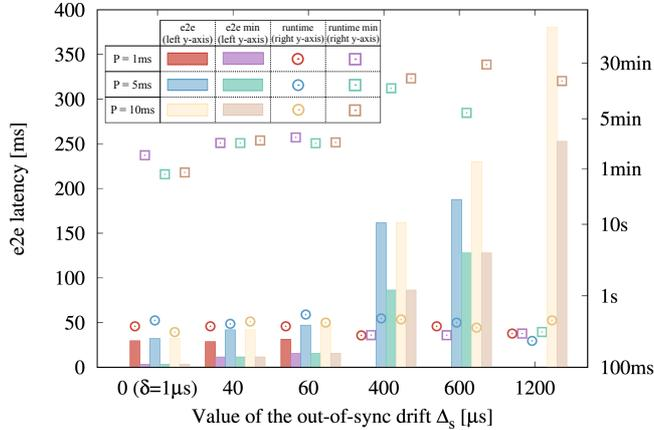
Figure 6. End-to-end latency with and without minimization objectives.
